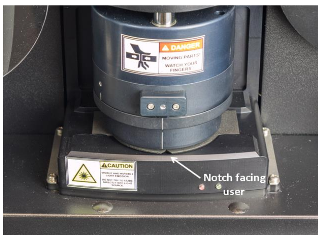
Figure 13. Calibration pad inserted beneath lifted optical chamber
