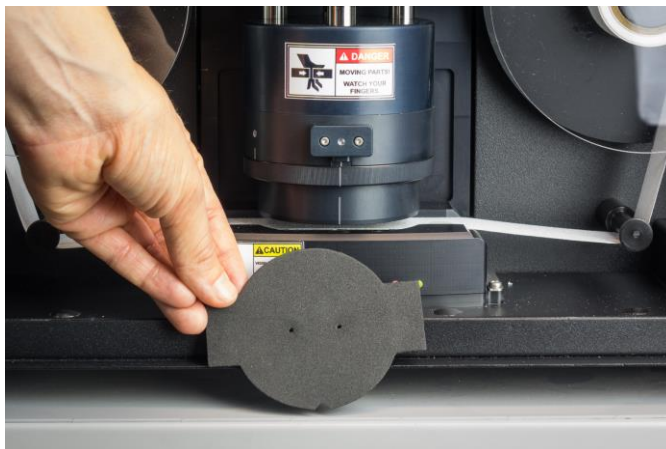
Figure 12. Insert calibration pad beneath the optical chamber with the notch facing out towards the user
