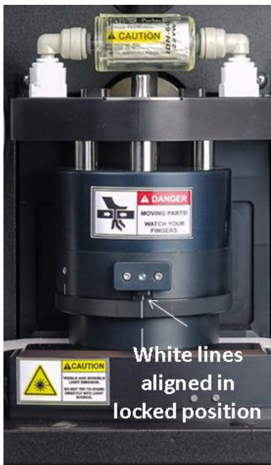
Figure 5. When the white lines on the optical chamber are aligned, the chamber is in locked position. Note that the optical chamber here is NOT yet lifted.
