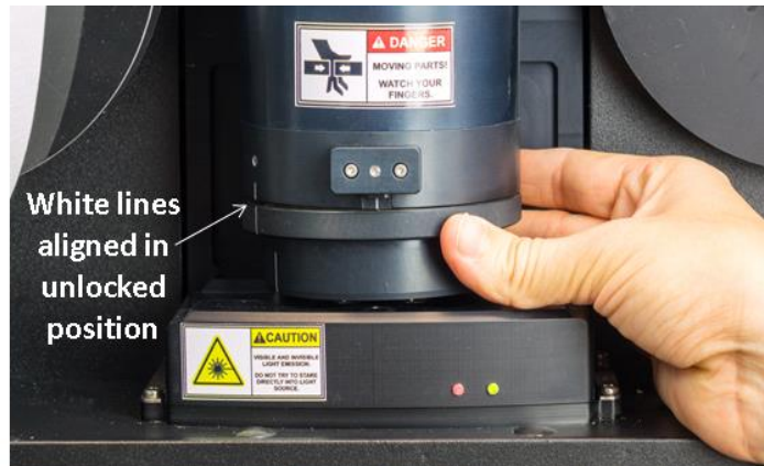
Figure 7. When white lines are aligned on the left, the bottom bayonet is loose and can be removed carefully
