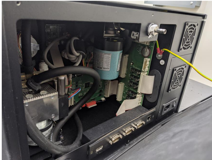
Figure 23. With the back panel open, the fuses are visible on the green panel.
