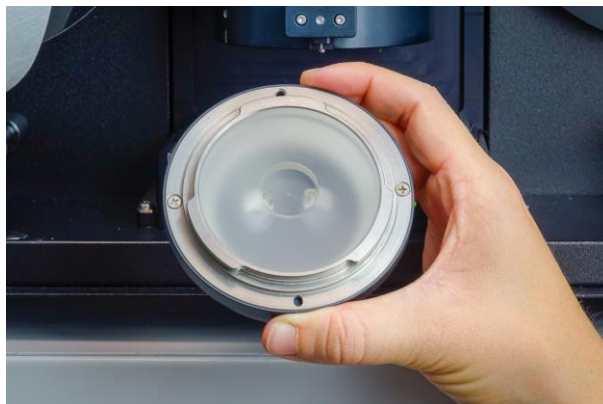
Figure 8. Inspect optical chamber for dust or debris
