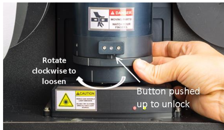
Figure 6. Push up button on front of optical chamber to unlock, then twist bottom bayonet clockwise to loosen
