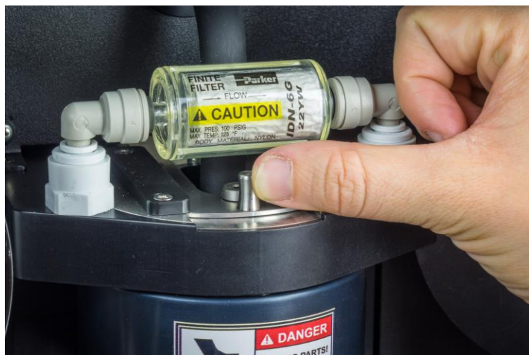
Figure 4. Push in metal latch to keep optical chamber locked in lifted position
