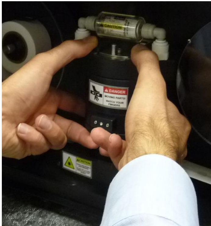
Figure 3. Squeeze the top and bottom of optical chamber once measurements are stopped to lift the optical chamber
