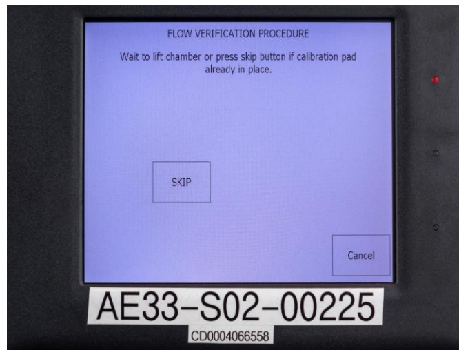
Figure 11. The instrument will prompt the user to insert the calibration pad
