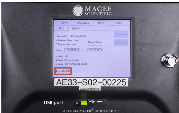
Figure 6. Files can be downloaded from the AE33 onto a USB stick by inserting a USB stick into the USB port on the front panel, and choosing 'ExportToUSB' in the DATA menu under the EXPORT tab
