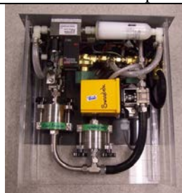
Top view of impactor box – mass flow controller is to left of HEPA filter at rear of impactor box.
