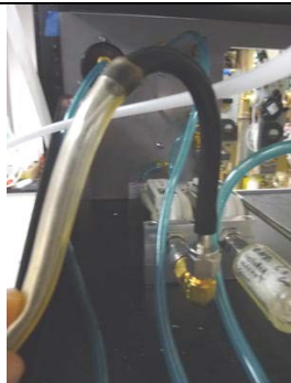
Flow calibration device is attached to inlet of TSI mass flow meter in CN box.
