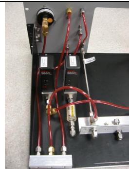
Top view of CN box with Brooks mass flow meters.
