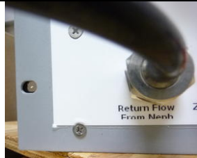
Flow calibration device is attached to back of impactor at port labeled 'return flow from neph'. You are calibrating the mass flow controller in the impactor box.
