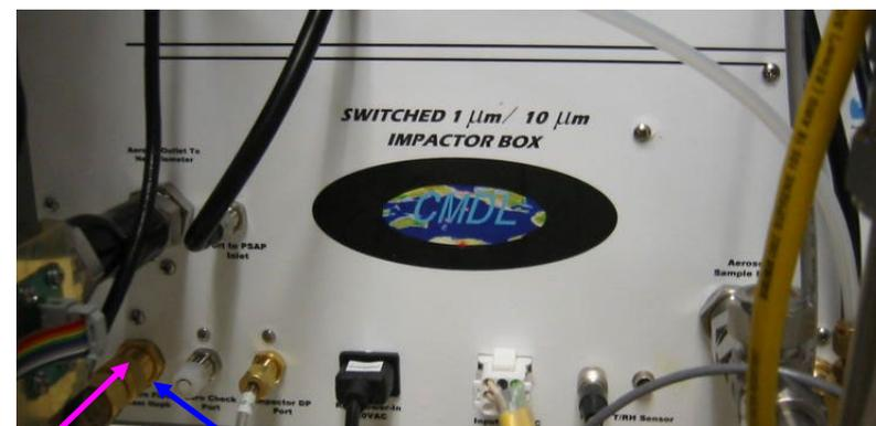
Connect flow meter to port labeled 'return flow from neph'. Flow controller and filter are in impactor box.
