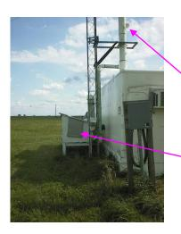
At BND, the sampling stack is cantilevered as at MLO and enters the trailer roof. The access port is easily accessible from the top of the trailer w/o climbing the tower. Excess stack flow is routed to the external pump box. BND has experienced some water leaks with the roof penetration inlet.
