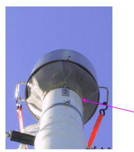
CPR is one of our most basic installations. The lab is a 6 ft x 8 ft wooden shack. The sampling stack is attached directly to the tower and the sampling lines enter the building from the flow – splitter through the side wall. Having the flow splitter outside the building requires more attention to check for leaks, corrosion, damage from winds, etc. The access port is easily accessible from the work platform.
