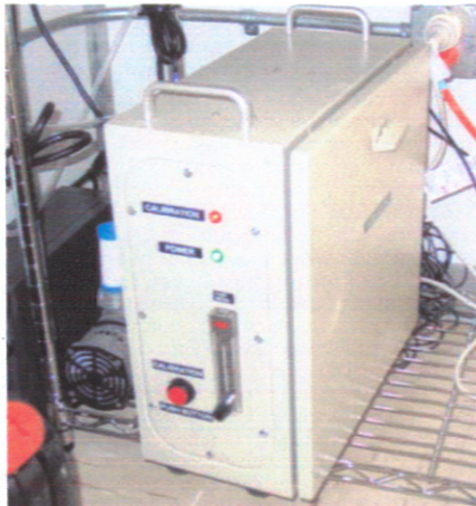
Figure 25: The Moody radon detector calibration unit.
