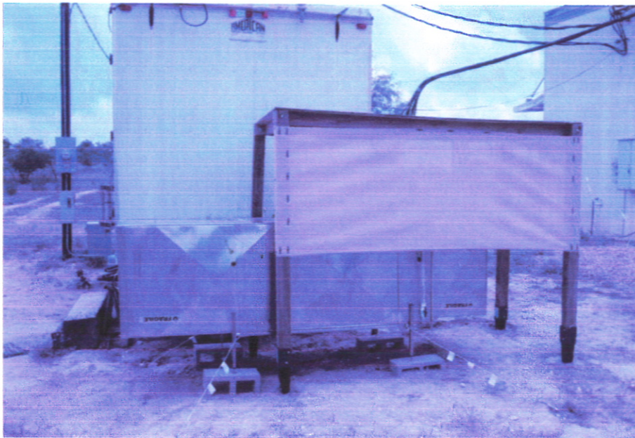
Figure 3: View from the south of the radon detector, its sun shade, and the instrument trailer.
