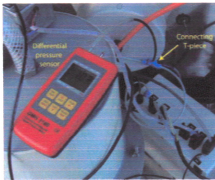
Figure 18: Calibration of the micro mass flow sensor with a hand held differential pressure sensor.
