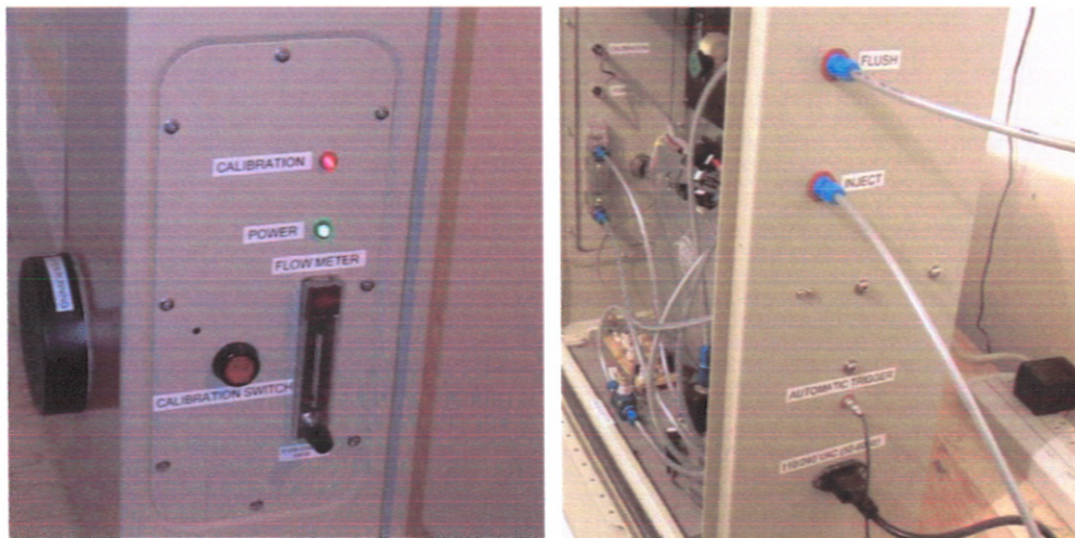
Figure 30: (a) Front and (b) rear views of a calibration unit similar to the one installed at the Moody tall tower site.
