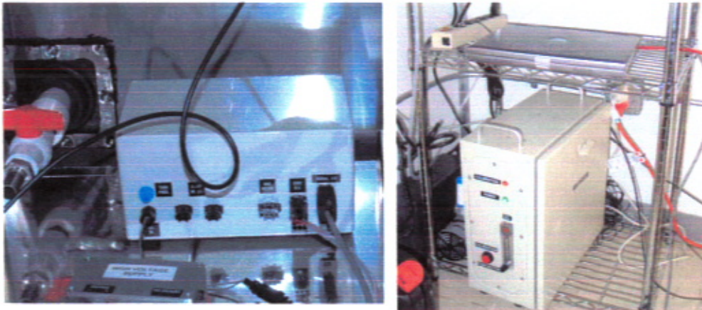
Figure 14: (a) Radon detector data logger, and (b) controlling computer and calibration unit.
