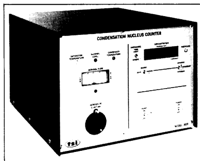
Figure 2. TSI Model 3020 Condensation Nucleus Counter.
