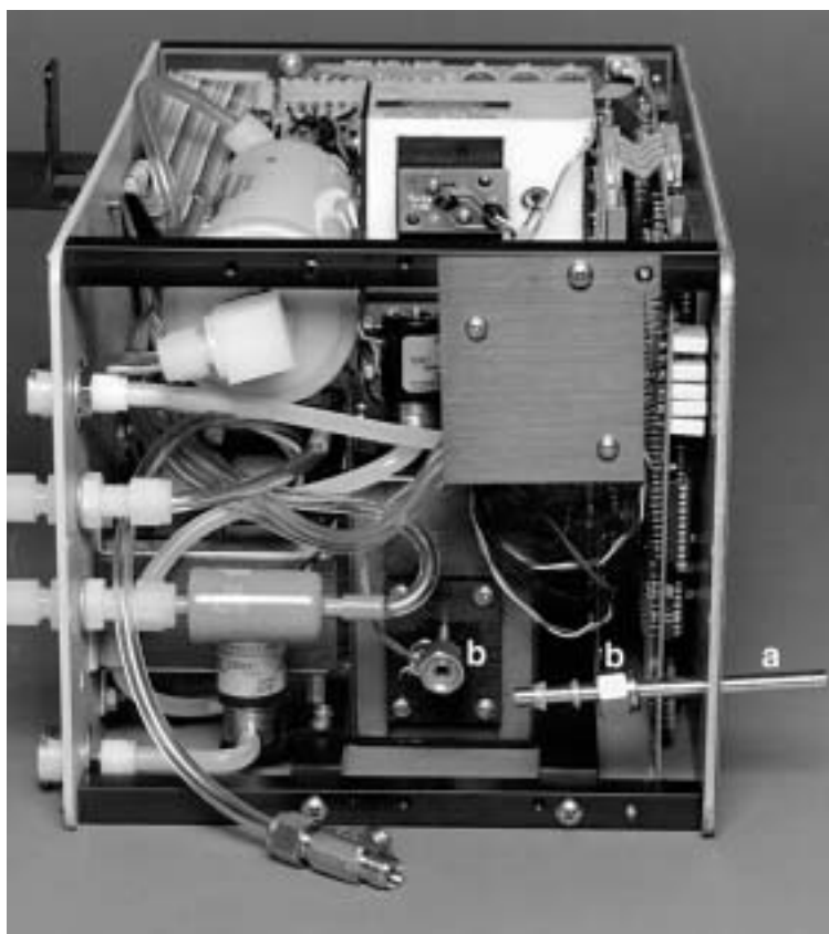
Figure 2-7 Removing the Front Inlet Tube; (a) Pull Inlet Tube Out; (b) Loosen Swagelok Nuts, 2 Places
