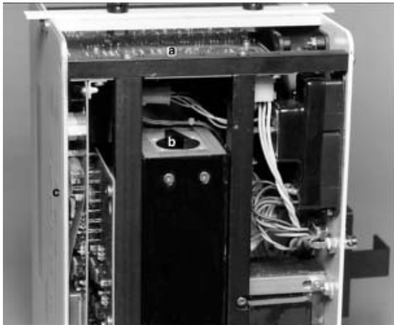
Figure 9-1 Locating the Filter Plug on the Bottom of the CPC: (a) Power Supply PC Board; (b) Filter Plug; (c) Front Panel
