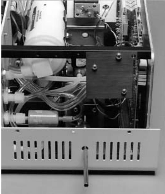
Figure 2-8d Side Inlet Option with the 2.8-in. Inlet Tube
