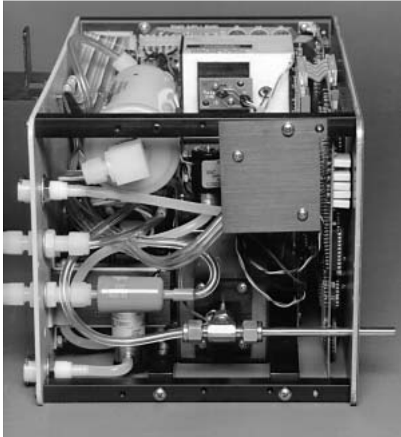
Figure 2-8b Front Inlet Option for Positioning the Inlet Tube
