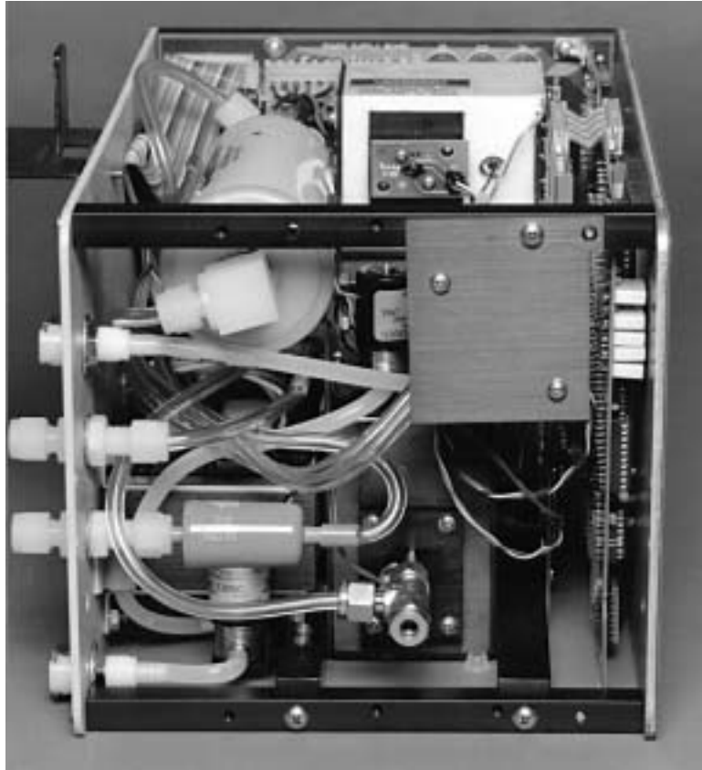
Figure 2-8c Side Inlet Option for Positioning the Inlet Tube
