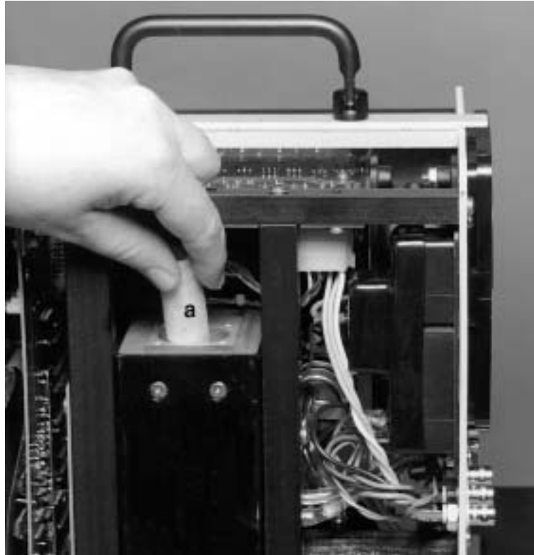
Figure 9-2 Replacing the Filter Tube: (a) Filter
