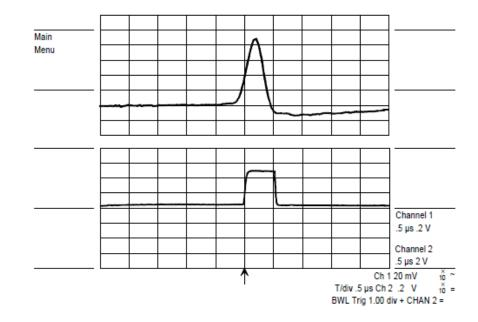
Figure 15. Pulse from TSI Manual Figure 6-2
