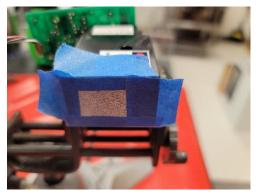
6. Using a standard pencil, make a rubbing to exactly outline the detector opening
