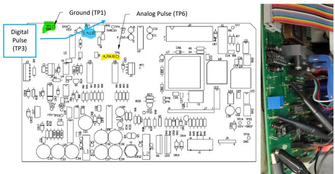
Figure 14. Z-Axis Adjustment Test Points
