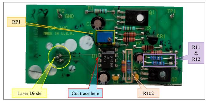
Figure 5. Component Side Rework
