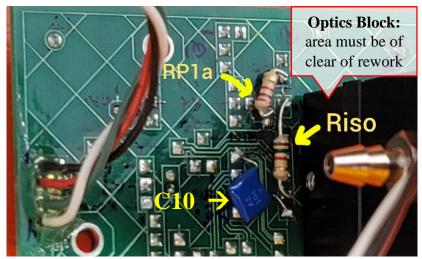
10. Check the resistance between PD (the new laser's photodiode, pin 3) and ground. Set RP1 so the impedance is near or at maximum (around 52 k $\Omega$ ). This sets the current to minimum for the later LD (laser diode) adjustment.
