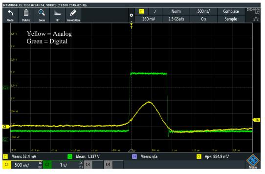
Figure 17. High Persistence Scope Capture Showing Signal Variation
