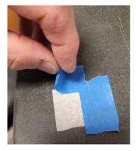
5. Pull the screen up and affix it over the center of the optics block detector hole.
