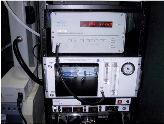
Top of instrument rack showing aethalometer, and CPC flow control box
