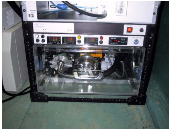
Bottom of instrument rack showing \mu mac (micromac) box, PID control box, and impactor box
