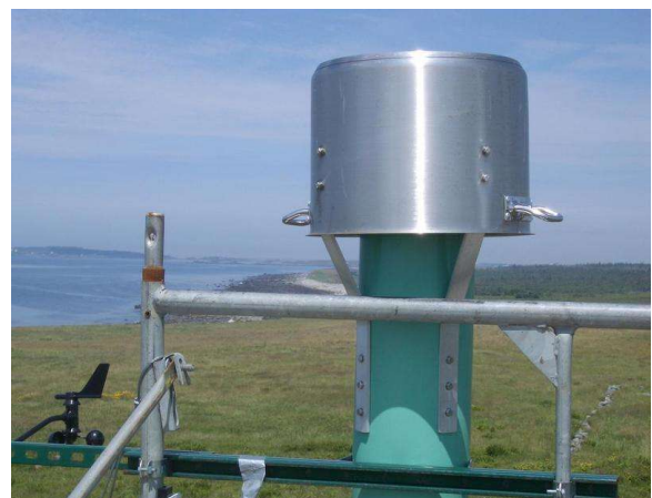
Figure 3-7: Stainless steel rain hat used at Chebogue Point, Canada, for an intensive field study. Aluminum brackets and a stainless steel cooking pot provide a simple and inexpensive solution.
