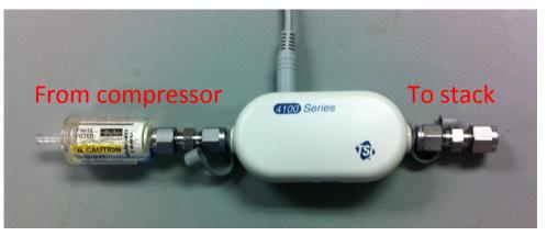
Install new flow meter. Note flow direction on bottom of flow meter. Connect tubing with filter to "inlet" and connect tubing to stack on "outlet". Plug in cable to flow meter.
