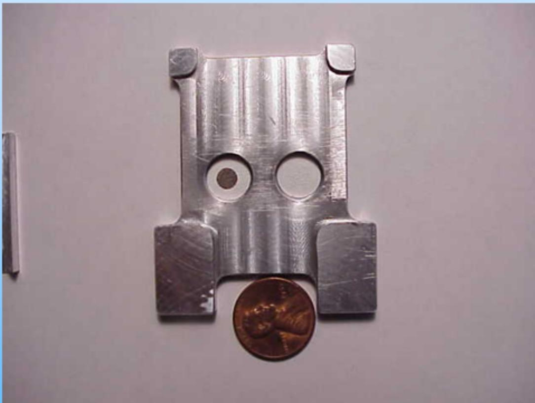
Particle-loaded filter on the left, reference filter on the right. Compare light transmission through these filters as a measure of light absorption
