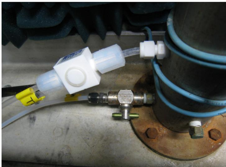
Figure 5. Sampling line connections of the BRW ozone instruments.
