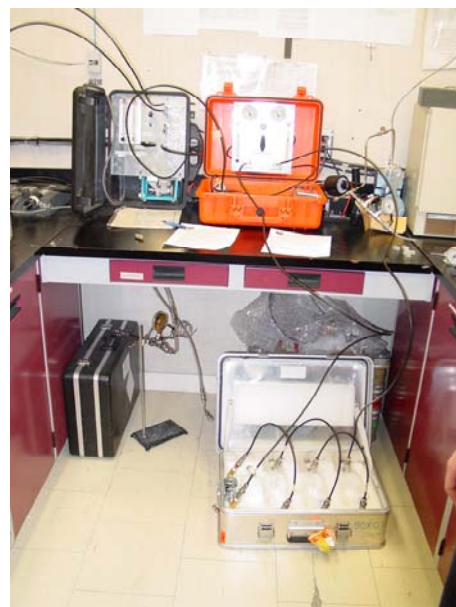
Figure 6: Photo showing the flask sampling apparatus from the Max-Planck Institute, Jena Germany. Sample air is drawn inside (from the top of a 10m tower) the laboratory using 3/8" Dekaron tubing.
