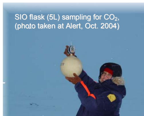
Figure 3: Photo showing the air sampling of a flask from the Scripps Institute of Oceanography. Sampling is conducted two hundred meters upwind of the laboratory.
