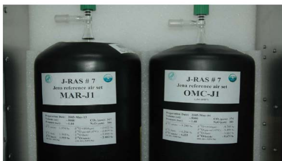
Figure 2: A JRAS-set comprises two 5L-glass flasks with artificial air at initially 1.6 Bar. The \text{CO}_2 in the flask air is produced from the MAR-J1 and OMC-J1 calcite powders.
