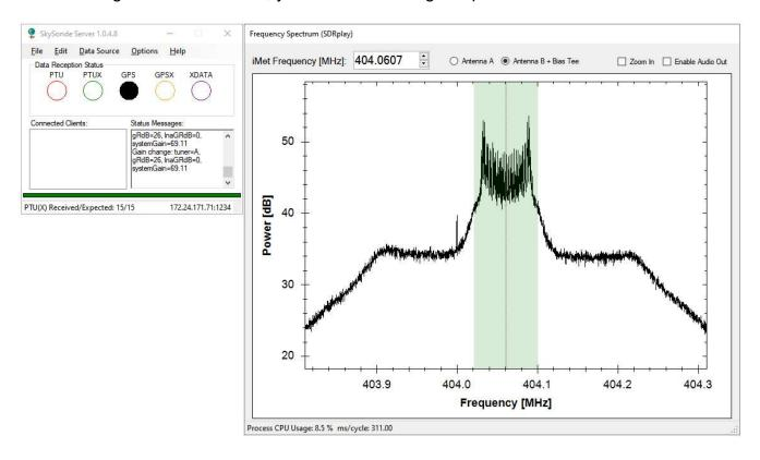
Try to center the signal spike within the shaded region, as shown. When setup properly, you will see radiosonde packets come through as blinking colored dots on the main window. It may take a few seconds for the SDR's auto gain control to get the correct amplification initially. **Narrowband radiosondes require more precise centering of the signal with the "Zoom In" option.**
