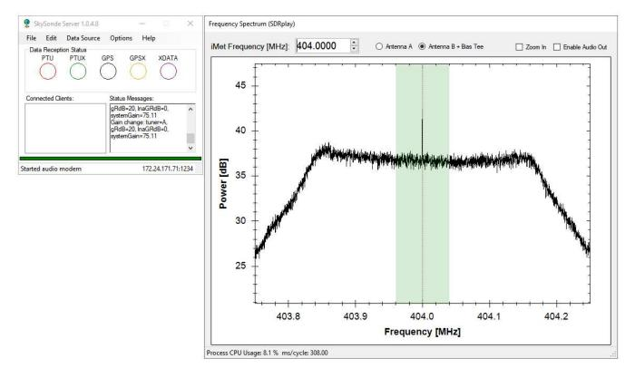
Make sure "Antenna B + Bias Tee" is selected (SDRplay RSP2/RSPdx only) when using an Uputronics preamp. Set the frequency to match the Intermet radiosonde by typing in a number to the "iMet Frequency" box and pressing enter. With no signal, you should see the flat plateau shape pictured above. The signal drops lower at the outer edges because of the hardware filter and a smoothing function the fourier transform algorithm uses.
