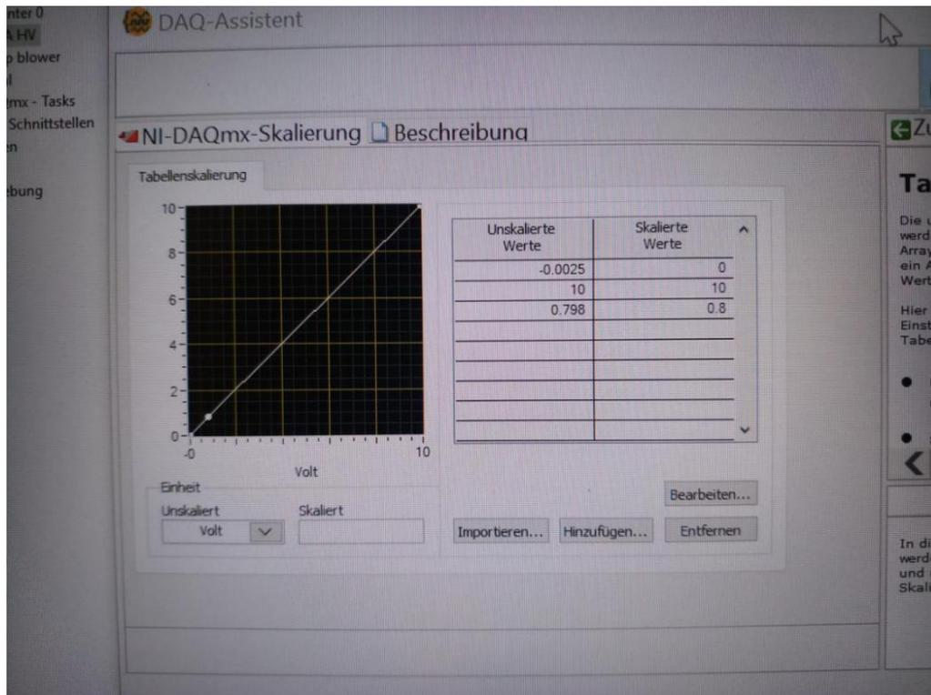
21. If the reading is greater than 5V then the scale (-0.0025) against 0 needs to be decreased by increasing the last digit or vis-versa.
