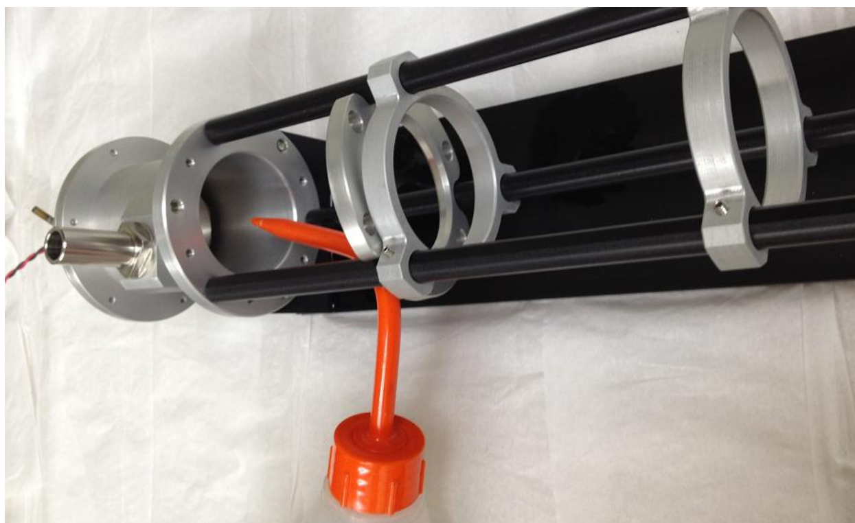
Figure 19: Rear mirror cleaning set-up
