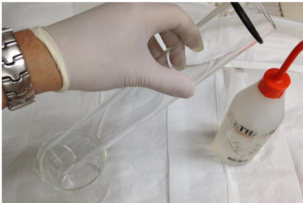
Figure 18: Glass tube cleaning set-up
