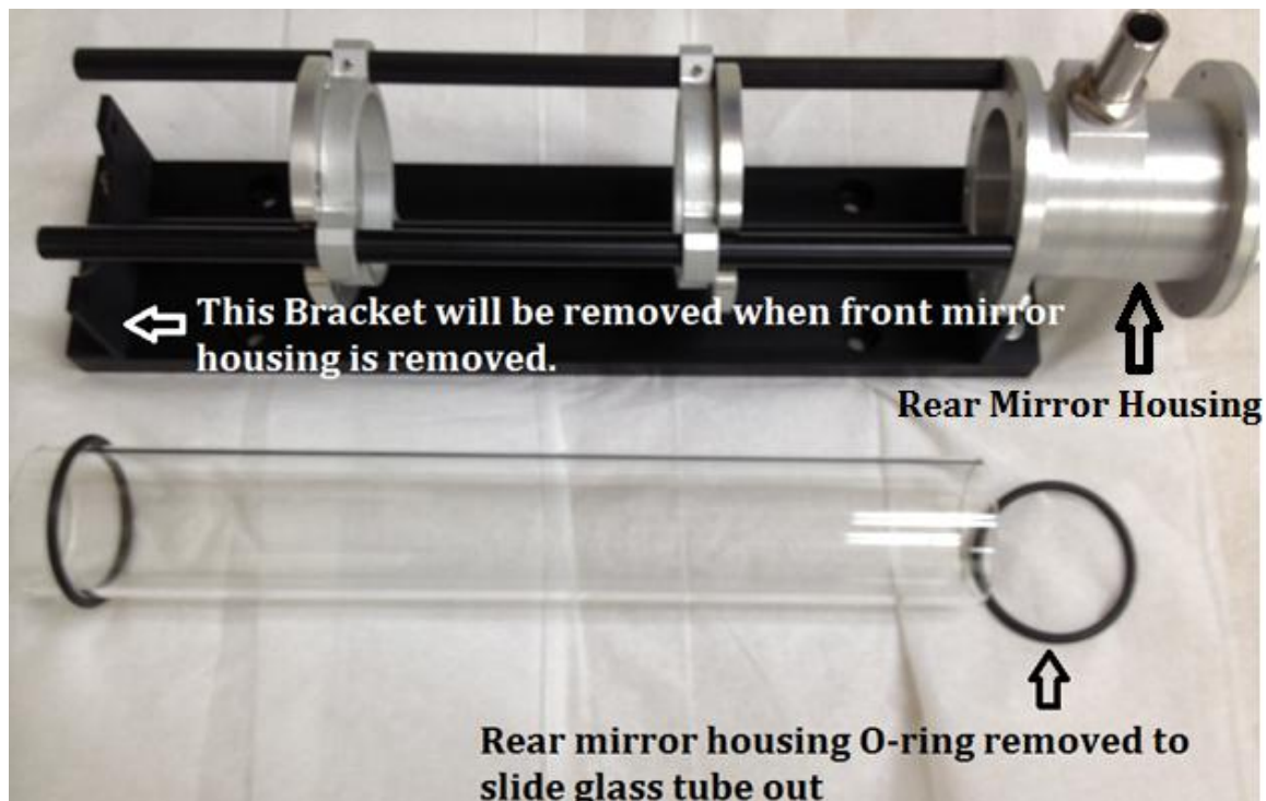
Figure 16: Removal of front mirror housing and glass tube
