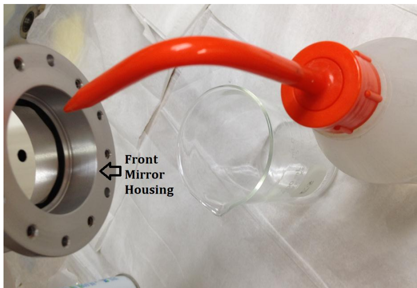
Figure 17: Front mirror cleaning set-up
