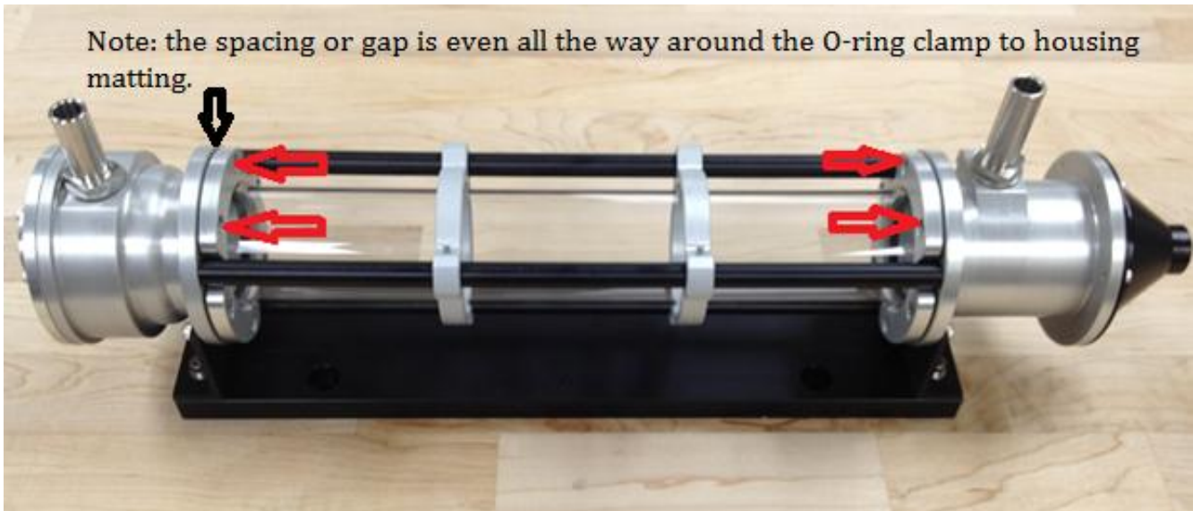
Figure 13: Retaining clamp gap note and location markers
