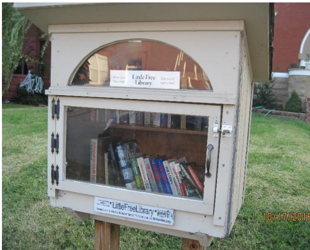
Figure 22. The LFLs differ as each is built around a recycled kitchen cabinet door and if there is recycled plastic sheets available, an extra viewing window is added at the top.
