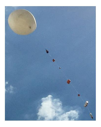
**Figure 1.** A dual-AirCore flight string launched by NOAA in California, USA.
