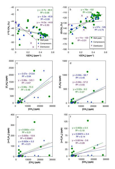
**Figure 1.** Composition of methane from natural gas sources in the Barnett Shale region. (a) Keeling plot of  $\delta^{13}$ C-CH<sub>4</sub> vs 1/[CH<sub>4</sub>]; (b)  $\delta$ D-CH<sub>4</sub> vs 1/[CH<sub>4</sub>]; (c) [C<sub>2</sub>H<sub>6</sub>] vs [CH<sub>4</sub>]; (d) [C<sub>3</sub>H<sub>8</sub>] vs [CH<sub>4</sub>]; (e) [n-C<sub>4</sub>H<sub>10</sub>] vs [CH<sub>4</sub>]; and (f) [n-C<sub>5</sub>H<sub>12</sub>] vs [CH<sub>4</sub>].
