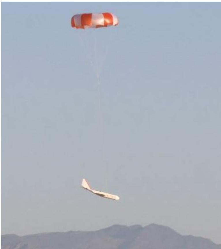
**Figure 1.** The NOAA HORUS platform equipped with AirCore scientific payload successfully completes a flight from 75,000 ft MSL at Edwards Air Force Base, CA.
