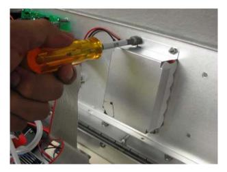
7. Place new Ni-MH battery on cover as shown below and connect it to charger circuit board
