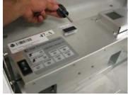
4. Disconnect battery pack from charger circuit board
