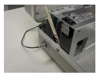
12. Charge the battery for 8 hours before collecting a sample. The charge light goes out when the battery is fully charged.
