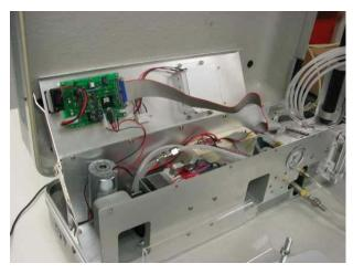
2. Remove cover from the electronics box inside the unit using a short Phillips head screwdriver
