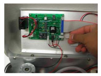
5. Remove 4 battery hold-down nuts using a 5/16" nut driver
