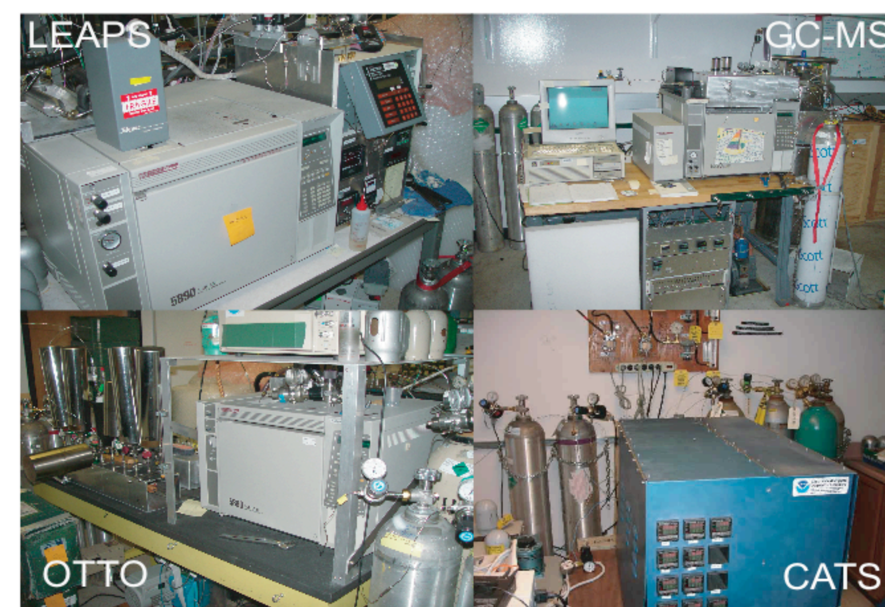
Fig. 3 Current NOAA/ESRL GC systems, Low Electrophilic Attachment Potential (LEAPS), GC-MS, and OTTO for analysis of flask samples in Boulder, Colorado (ESRL), and the in situ Chromatograph for Atmospheric Trace Species (CATS) at five baseline observatories (Mauna Loa GC pictured here).
