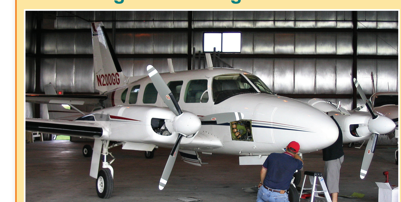
A small two-engine aircraft is equipped by USA's National Oceanic and Atmospheric Administration for measurements of greenhouse gases.
