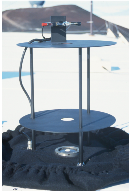
Figure 2.16. Calibration stand with a 200-Watt lamp mounted on top of a SUV-100 spectroradiometer. The lamp power is connected to the roofbox immediately below the fixture. Baffles limit stray light. During operation, an internally-blackened barrel is placed over this fixture.
