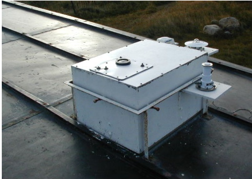
Figure 3.4.1. SUV-100 spectroradiometer installed in the roof of the CADIC facility in Ushuaia.
