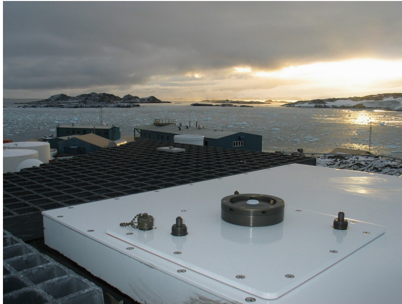
Figure 3.2.2. Installation of SUV-100 spectroradiometer at Terra Lab. The main buildings of Palmer Station are in the background.
