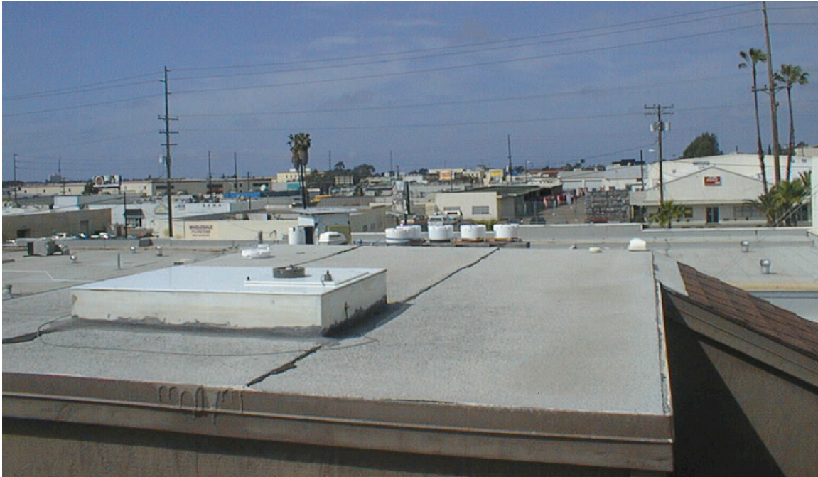
Figure 3.5.1. SUV-100 mounted through the roof of a specially constructed room at Biospherical Instruments in San Diego, California. This rooftop facility is used for calibration and intercomparison of UV and visible radiometers.
