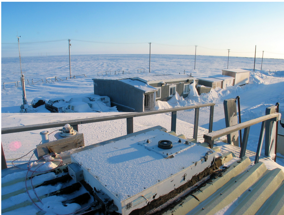
Figure 3.6.1. Roof installation of the SUV-100 spectroradiometer in Barrow with snow-covered tundra in the background.
