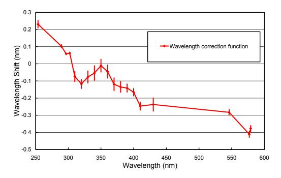
**Figure 5.1.7.** Monochromator non-linearity correction functions for McMurdo 2003/04 data. The function was calculated with the Fraunhofer-correlation method.
