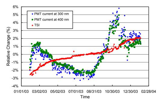
**Figure 5.1.3.** *Time-series of PMT current at 300 and 400 nm, and TSI signal during measurements of the internal irradiance reference lamp during the McMurdo 2003/04 season. The data is normalized to the average value of the whole season.*
