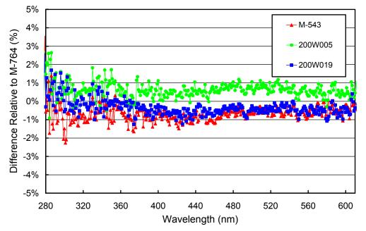
**Figure 5.1.1.** Comparison of McMurdo lamps M-543, 200W005, and 200W019 with the BSI traveling standard M-764 at the beginning of the season (1/27/03).
