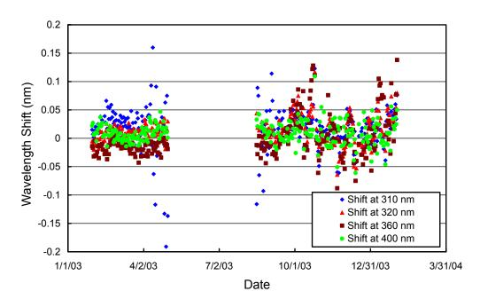
**Figure 5.1.8.** Check of the wavelength accuracy of the final data at four wavelengths by means of Fraunhofer correlation. The noontime measurement has been evaluated for each day of the season. No correlation data is available during the polar night.
