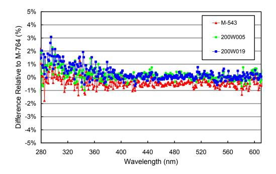
**Figure 5.1.2.** Comparison of McMurdo lamps M-543, 200W005, and 200W019 with the BSI traveling standard M-764 at the end of the season (2/2/04).
