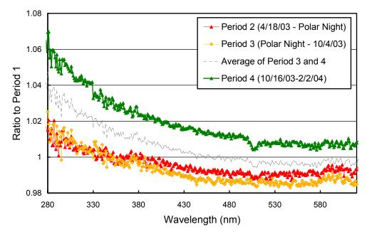
Figure 5.1.4 Ratio of irradiance assigned to the internal reference lamp to the Period 1, 1/29/03–4/17/03.
