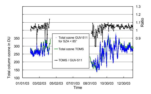
**Figure 5.1.11.** Comparison of total column ozone measurements from GUV-511 and NASA/TOMS Earth Probe satellite. GUV-511 measurements are plotted in 15 minute intervals. For calculating the ratio of both data sets, only GUV-511 measurements coincident with the TOMS overpass data were evaluated.
