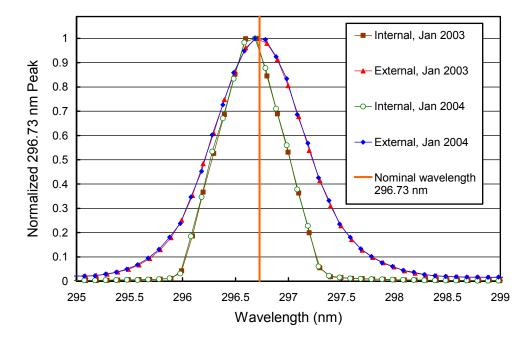
**Figure 5.1.9** The 296.73 mercury line as registered by the PMT from external and internal sources. The wavelength scale is the same as applied for solar measurements, i.e., it is based on a combination of internal scans and the Fraunhofer-correlation method. It is assumed that the wavelength registration of the monochromator did not shift between internal and external scans, which were close in time.
