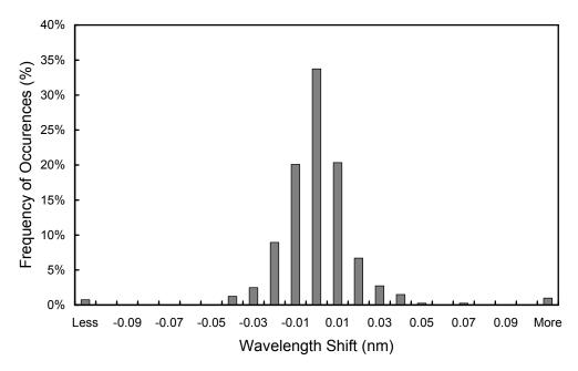
Figure 5.3.6. Frequency distribution of the difference of the measured position of the 296.73 nm mercury line between consecutive wavelength scans. The x-labels give the center wavelength shift for each column. The 0-nm histogram column covers the range -0.005 to +0.005 nm. "Less" means shifts beyond -0.105 nm; "more" means shifts beyond +0.105 nm.
