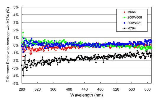
**Figure 5.3.1.** Comparison of South Pole lamps 200W006, 200W021, and M-666 and the BSI traveling standard M-764 at the start of the season (1/21/05). The calibration functions of lamps M-666 and 200W021 are based on comparisons with the traveling standard 200W017, which were performed in January 2006.
