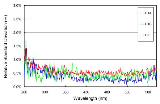
**Figure 5.3.5.** Relative standard deviation calculated from the absolute calibration scans measured during the South Pole 2005/06 season.
