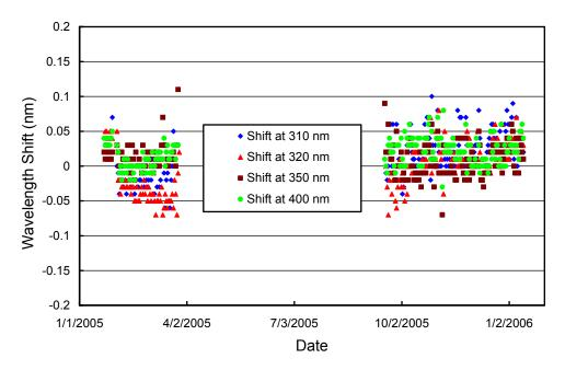
**Figure 5.3.8.** Wavelength accuracy check of the final data at four wavelengths by means of Fraunhofer correlation. The noontime measurement has been evaluated for each day of the season. No data exist during Polar Night.
