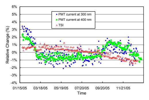
**Figure 5.3.3.** Time-series of PMT current at 300 and 400 nm, and TSI signal during measurements of the internal irradiance standard performed during the South Pole 2005/06 season. The data are normalized to the average of the whole period.
