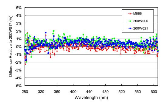
**Figure 5.3.2.** Comparison of South Pole lamps 200W006, 200W021, and M-666 with the BSI traveling standard 200W017 at the end of the season (1/14/06).
