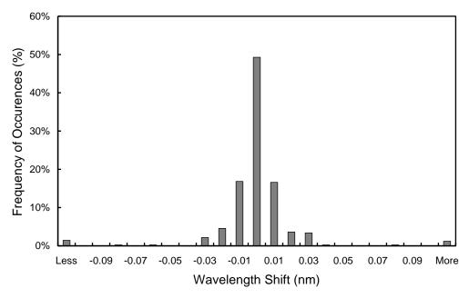
**Figure 5.3.7.** Frequency distribution of the difference of the measured position of the 296.73 nm mercury line between consecutive wavelength scans. The x-labels give the center wavelength shift for each column. The 0-nm histogram column covers the range -0.005 to +0.005 nm. "Less" means shifts beyond -0.105 nm; "more" means shifts beyond +0.105 nm.
