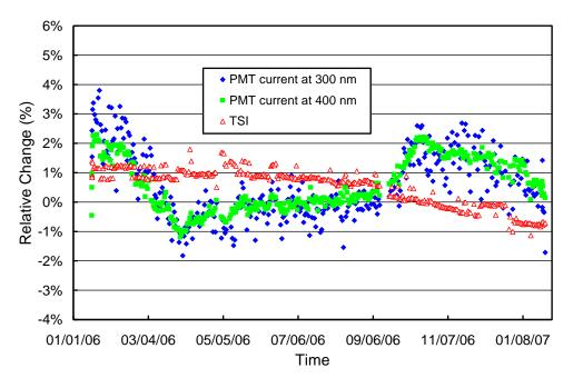
**Figure 5.3.3.** Time-series of PMT current at 300 and 400 nm, and TSI signal for measurements of the internal irradiance standard performed during the South Pole 2006/07 season. Data are normalized to the average of the whole period.
