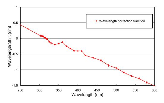
Figure 5.3.8. Monochromator non-linearity correction function for the South Pole 2006/07 season.
