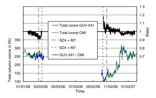
**Figure 5.3.12.** Comparison of total column ozone measurements from GUV-541 and OMI. GUV-541 measurements are plotted in 15 minute intervals. For calculating the ratio of both data sets, only GUV-541 measurements concurrent with OMI overpass data were evaluated.
