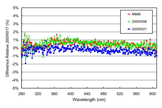
**Figure 5.3.1.** Comparison of South Pole lamps 200W006, 200W021, and M-666 with BSI traveling standard 200W017 at the start of the season (1/17/06–1/18/06).
