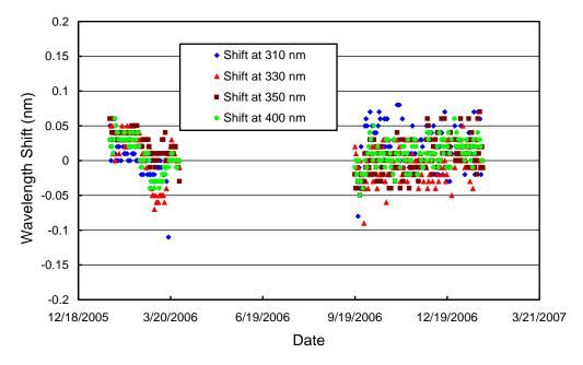
**Figure 5.3.9.** Wavelength accuracy check of final data at four wavelengths by means of Fraunhofer correlation. Measurement performed at 00:00 UT were evaluated for each day of the season. No data exist during Polar Night.
