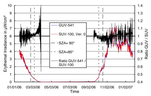
**Figure 5.3.11.** Comparison of erythemal irradiance measured by the SUV-100 spectroradiometer and the GUV-541 radiometer. SUV-100 measurements are based on "Version 0" (cosine-error uncorrected) data.
