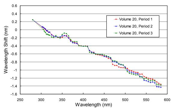
Figure 5.3.4. Monochromator non-linearity correction functions for the South Pole 2010/11 season.
