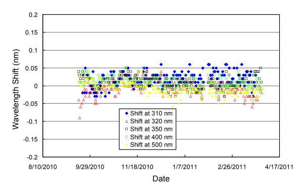
**Figure 5.3.5.** Wavelength accuracy check of final data at four wavelengths by means of Fraunhofer-line correlation. Measurement performed at 00:00 UT were evaluated for each day of the season. No data exist during Polar Night.
