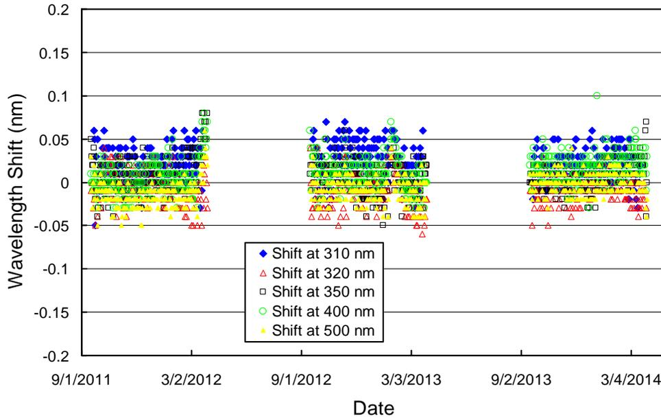
**Figure 5.3.5.** Wavelength accuracy check of final data at five wavelengths by means of Fraunhofer-line correlation. Measurement performed at 00:00 UT were evaluated for each day of the reporting period. No data exist during Polar Night.
