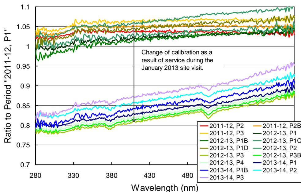
**Figure 5.3.3.** Ratios of spectral irradiance assigned to the internal lamp relative to Period "2011-12, P1".
