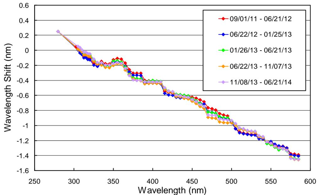
**Figure 5.3.4.** Monochromator non-linearity correction functions for South Pole data of the period 9/1/11 - 6/21/14.
