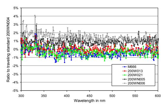
**Figure 3.1.** Comparison of South Pole lamps M-666, 200W021, 200W013, 200WN005, and 200WN006 with traveling standard 200W004 at the beginning of the January 2015 site visit.
