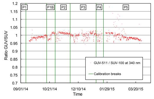
**Figure 3.2.** Ratio of GUV-541 #29239 measurements (340 nm channel) with SUV-100 measurements. SUV-100 data were weighted with the spectral response function of this GUV channel. The vertical lines indicate times when the calibration applied to SUV-100 data was changed (see also Table 3.1).
