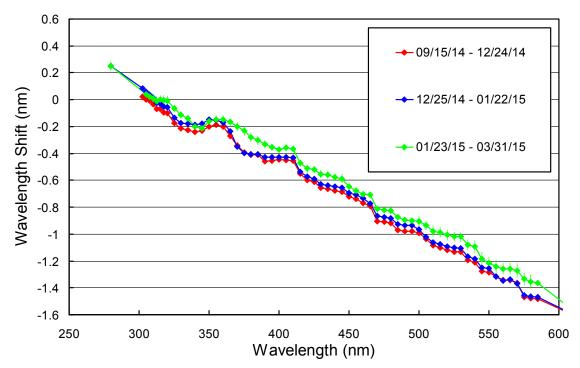
**Figure 3.4.** Monochromator non-linearity correction functions for South Pole data of the period 9/15/14 - 3/31/15.
