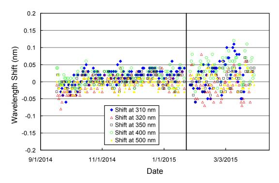
**Figure 3.5.** Wavelength accuracy check of final data at five wavelengths by means of Fraunhofer-line correlation. Measurement performed at 00:00 UT were evaluated for each day of the reporting period. The vertical line indicates the time of the site visit.
