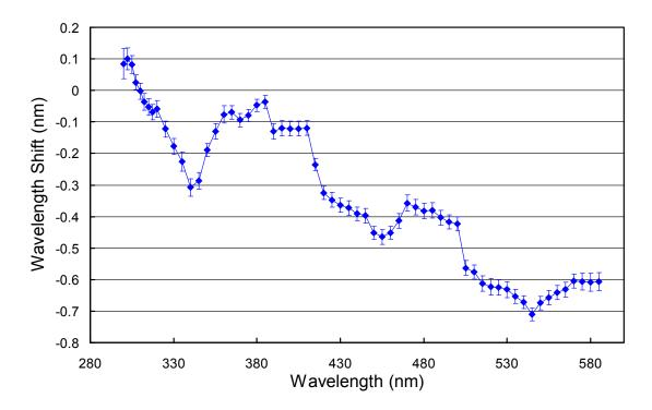
Figure 5. Monochromator mapping function.
