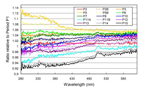
**Figure 3.** *Ratios of spectral irradiance assigned to the internal reference lamp for periods P2 – P15 relative to Period P1. Broken lines indicate interpolated data.*
