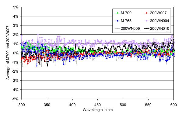
**Figure 1.** Comparison of the calibration of on-site standards M700, 200W007, M765, 200WN009, and 200WN010; and the traveling standard 200WN004 on 3/28/2015. Data are reference to the average of the measurements of lamps M700 and 200W007.
