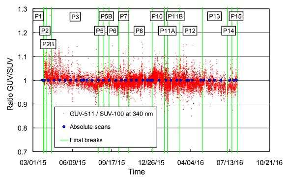
**Figure 4.** *Ratio of GUV-511 measurements at 340 nm with final SUV-100 measurements. The latter were weighted with the spectral response function of the GUV-511 340 nm channel.*
