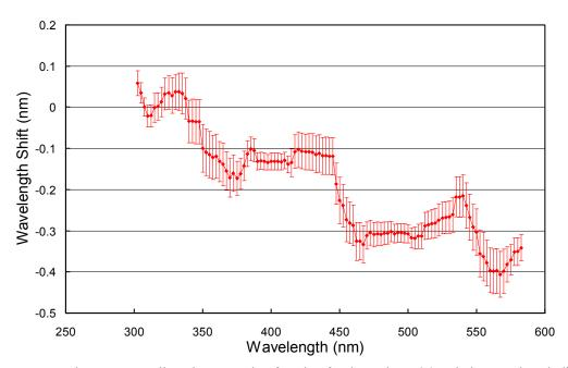
**Figure 5.** Monochromator non-linearity correction function for the Volume 26 period. Error bars indicate the 1σ-variation.
