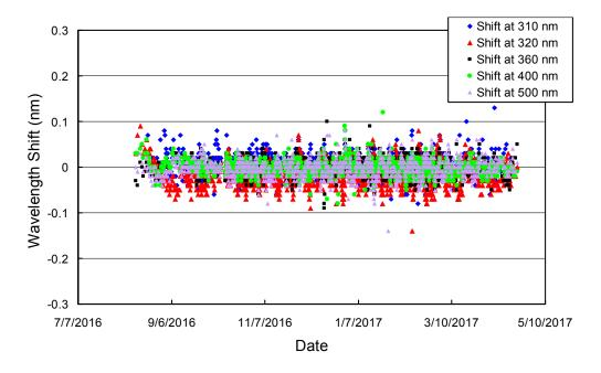
**Figure 7.** Check of the wavelength accuracy of <u>Version 2</u> data at six wavelengths by means of Fraunhofer-line correlation. The plot is based on hourly measurements.
