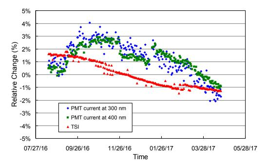
**Figure 2.** Measurements of the SUV-100's TSI sensor and PMT currents at 300 and 400 nm. Data are shown as relative change.
