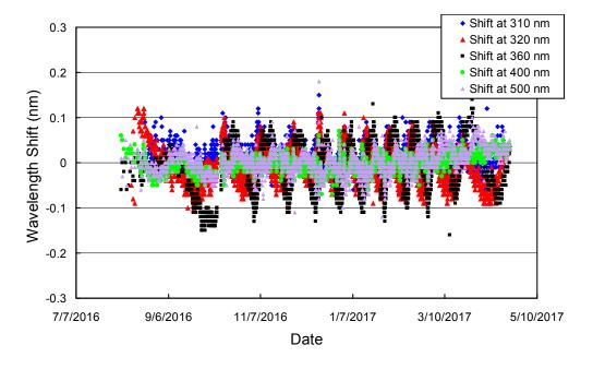
**Figure 6.** Check of the wavelength accuracy of <u>Version 0</u> data at six wavelengths by means of Fraunhofer-line correlation. The plot is based on hourly measurements.
