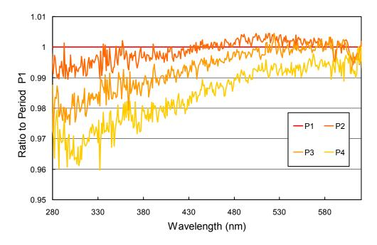
**Figure 2.** Ratios of spectral irradiance assigned to the internal reference lamp during Periods P2 through P4, relative to Period P1.
