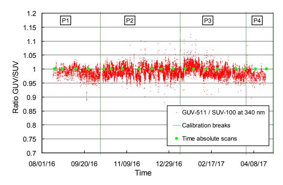
**Figure 3.** Ratio of GUV-511 (340 nm channel) and SUV-100 measurements. Green vertical lines indicate times when the SUV-100 calibration was changed. The times when "absolute" calibration scans of the SUV were performed are also indicated.
