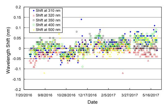
**Figure 6.** Wavelength accuracy check of the final Version 0 data at five wavelengths by means of Fraunhofer-line correlation. Noontime measurements from every day of the year have been evaluated.
