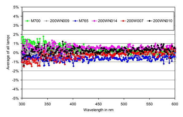
**Figure 1.** Comparison of the calibration of on-site standards M700, 200W007, M765, 200WN009, and 200WN010; and the traveling standard 200WN014 on 4/4/2017. Data are reference to the average of the measurements of all lamps.
