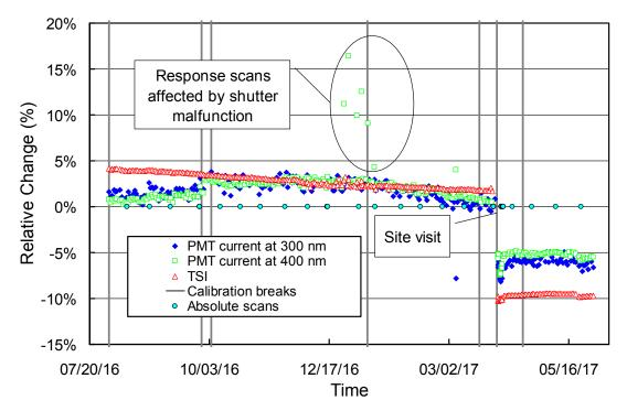
**Figure 2.** Time-series of PMT current at 300 and 400 nm, and TSI signal. All data were extracted from measurements of the internal irradiance standard and are normalized to their average. Calibration break points (Table 1) and times of absolute scans are also indicated. The response lamp that was installed during the site visit burns darker, explaining the difference in pre- and post-visit measurements.
