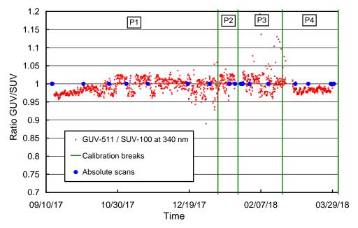
**Figure 3.2.** Ratio of GUV-541 S/N 29239 measurements (340 nm channel) with SUV-100 measurements. SUV-100 data were weighted with the spectral response function of this GUV channel. The vertical green lines indicate times when the calibration applied to SUV-100 data was changed (see also Table 3.1).
