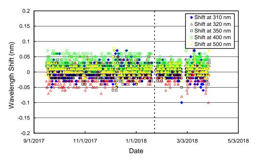
**Figure 3.6.** Wavelength accuracy check of <u>Version 2</u> data at five wavelengths by means of Fraunhofer-line correlation. The vertical broken line indicates the time of the site visit.
