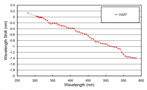
**Figure 3.4.** *Monochromator non-linearity correction function.*
