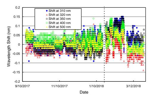
**Figure 3.5.** Wavelength accuracy check of <u>Version 0</u> data at five wavelengths by means of Fraunhofer-line correlation. The vertical broken line indicates the time of the site visit.
