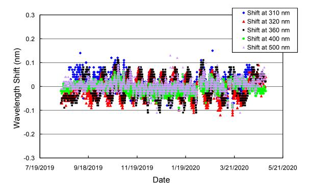
**Figure 6.** Check of the wavelength accuracy of <u>Version 0</u> data at six wavelengths by means of Fraunhofer-line correlation. The plot is based on hourly measurements.
