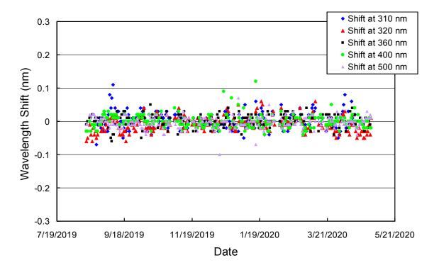
**Figure 7.** Check of the wavelength accuracy of <u>Version 2</u> data at six wavelengths by means of Fraunhoferline correlation. The plot is based on measurements at 01:00 UT (approximate local solar noon at McMurdo).
