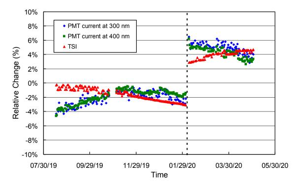
**Figure 2.** Measurements of the SUV-100's TSI sensor and PMT currents at 300 and 400 nm. Data are shown as relative change and normalized to the average of the entire period. The broken vertical line indicates the time when the internal lamp was changed during the site visit.
