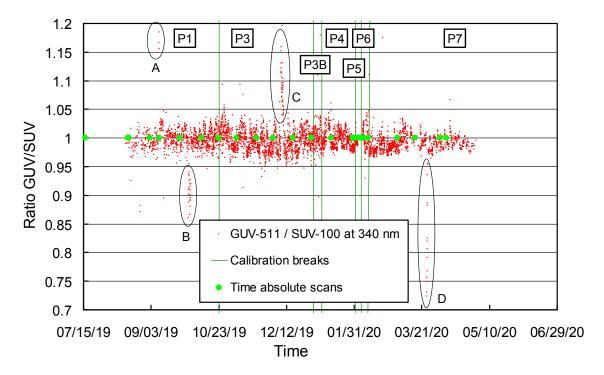
**Figure 4.** Ratio of GUV-511 (340 nm channel) and SUV-100 measurements. Green vertical lines indicate times when the SUV-100 calibration was changed. The times when "absolute" calibration scans of the SUV-100 were performed are also indicated. Periods with outliers are marked with ellipses and discussed in the text.
