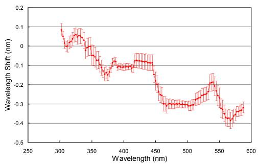
**Figure 5.** Monochromator non-linearity correction function for the Volume 29 period. Error bars indicate the  $1\sigma$ -variation.
