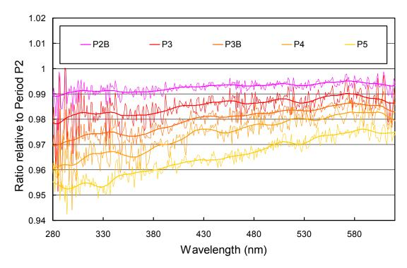
**Figure 3.4.** *Ratios of spectral irradiance assigned to the internal lamp relative to the spectral irradiance of Period P2.Thin lines indicate the actual ratio; thick lines indicate smoothed ratios. Calibrations functions are based on the latter.*
