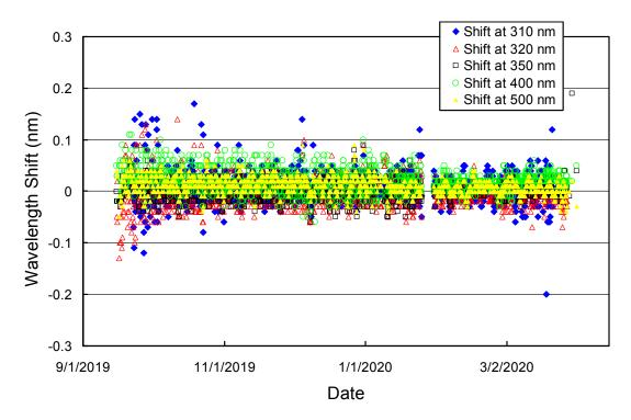
**Figure 3.7.** Wavelength accuracy check of <u>Version 2</u> data at five wavelengths by means of Fraunhoferline correlation.
