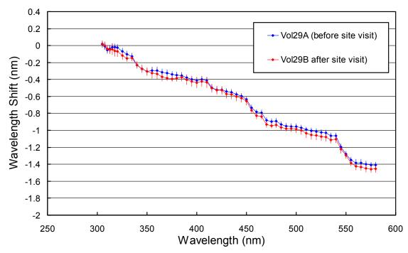
Figure 3.5. Monochromator non-linearity correction functions.
