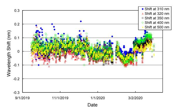
**Figure 3.6.** Wavelength accuracy check of <u>Version 0</u> data at five wavelengths by means of Fraunhoferline correlation.
