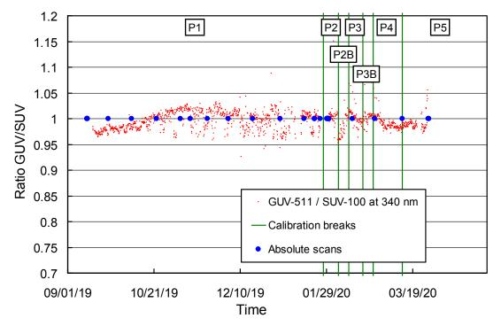
**Figure 3.3.** *Ratio of GUV-541 (S/N 29239) measurements (340 nm channel) with SUV-100 measurements. SUV-100 data were weighted with the spectral response function of this GUV channel. The vertical green lines indicate times when the calibration applied to SUV-100 data was changed (see also Table 3.1).*
