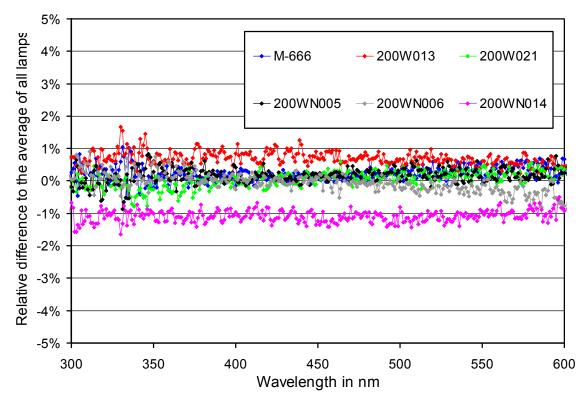
*Figure 3.1.* Comparison of South Pole lamps M-666, 200W021, 200W013, 200WN005 and 200WN006, and traveling standard 200WN014 based absolute scans performed at the end of the site visit, on 29 and 30 January 2020.
