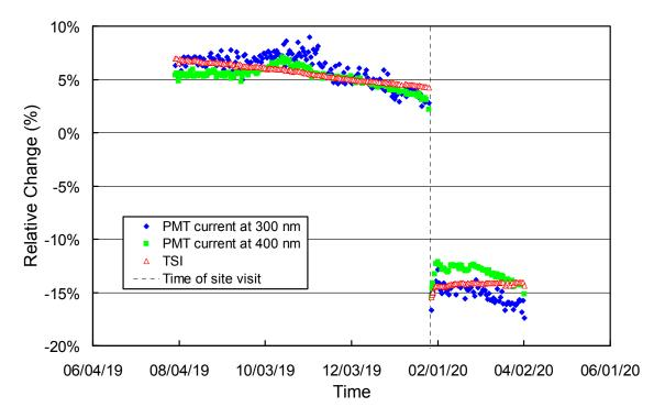
*Figure 3.2. Time-series of PMT current at 300 and 400 nm, plus the TSI signal, derived from daily measurements of the SUV-100's the internal irradiance standard. Data are normalized to the average of the whole period.*
