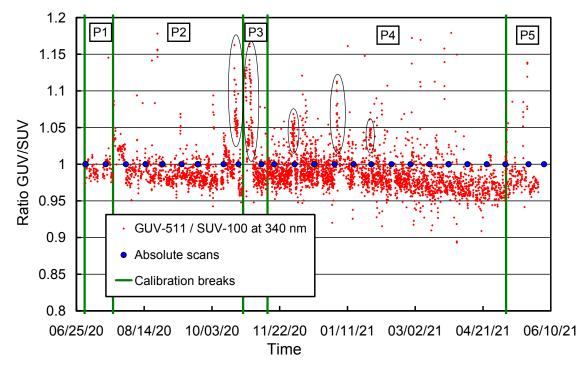
**Figure 4.** Ratio of GUV-511 measurements at 340 nm with SUV-100 measurements. The latter were weighted with the spectral response function of the GUV-511's 340 nm channel. Narrow clusters of vertical data points marked by ellipses are likely caused by snow covering the SUV-100 collector.
