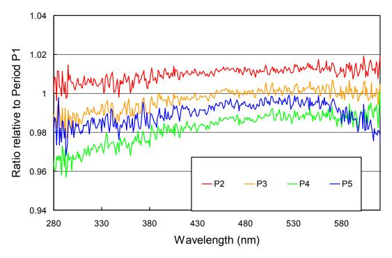
**Figure 3.** Ratios of spectral irradiance assigned to the internal reference lamp for periods P1 - P7, relative to Period P1.
