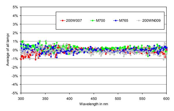
**Figure 1.** Comparison of the calibration of on-site standards 200W007, M700, and M765 with long-term standard 200WN009 on 9/22/2020.
