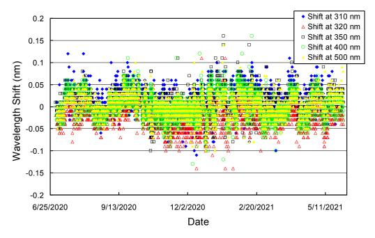
**Figure 6.** Wavelength accuracy check of the final <u>Version 0</u> data at five wavelengths by means of Fraunhofer-line correlation. Measurements were evaluated in four-hour increments.
