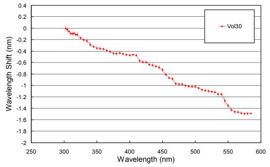
Figure 3.5. Monochromator non-linearity correction functions.
