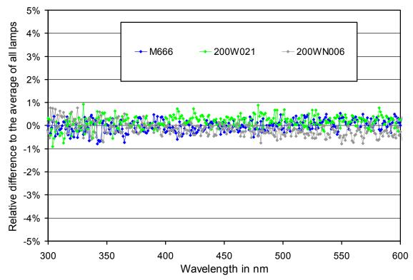
*Figure 3.1.* Comparison of South Pole lamps M-666, 200W021, and 200WN006 based absolute scans performed on 10 September 2020.
