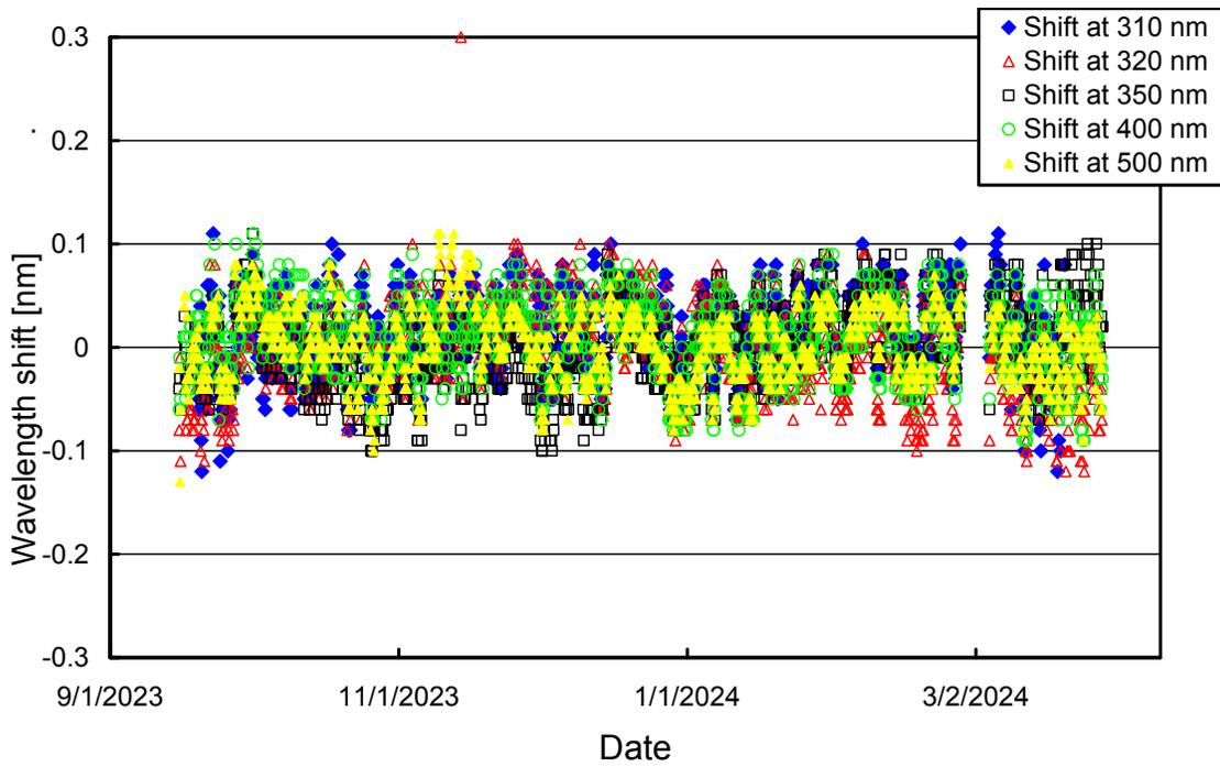
Figure 5. Wavelength accuracy check of Version 0 data at five wavelengths by means of Fraunhofer-line correlation.
