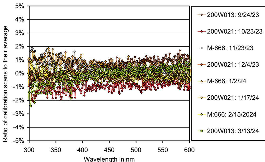
**Figure 1.** Comparison calibration scans of South Pole working standard M-666, 200W021, and 200W013 during the reporting period.
