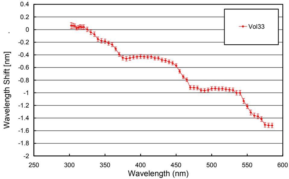
Figure 4. Monochromator non-linearity correction functions.
