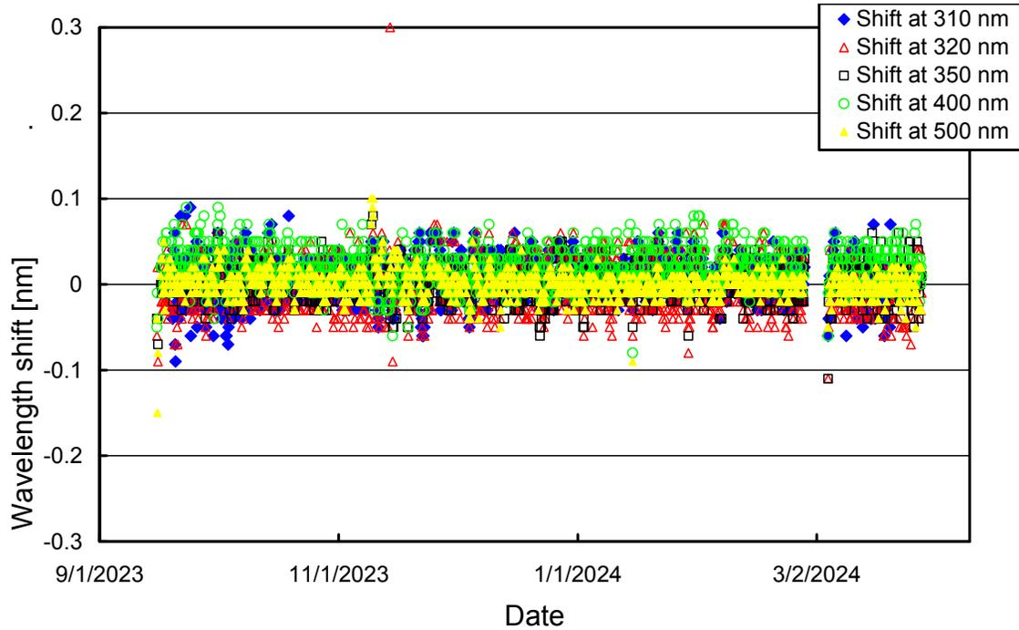
**Figure 6.** Wavelength accuracy check of *Version 2* data at five wavelengths by means of Fraunhofer-line correlation.
