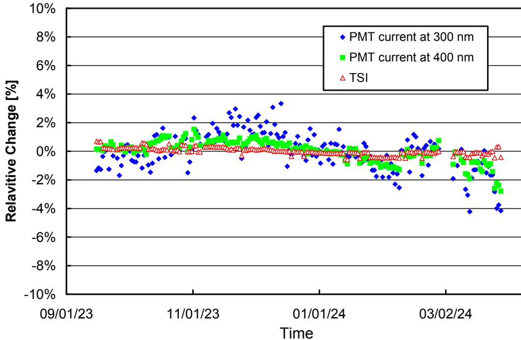
**Figure 2.** Time-series of PMT current at 300 and 400 nm, plus the TSI signal, derived from daily measurements of the SUV-100's the internal irradiance standard. Data are normalized to the average of the whole period.
