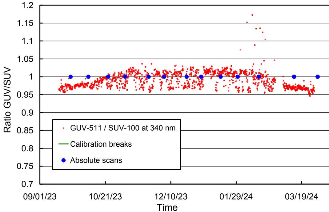
**Figure 3.** Ratio of GUV-541 (S/N 29239) measurements (340 nm channel) with SUV-100 measurements. SUV-100 data were weighted with the spectral response function of this GUV channel.
