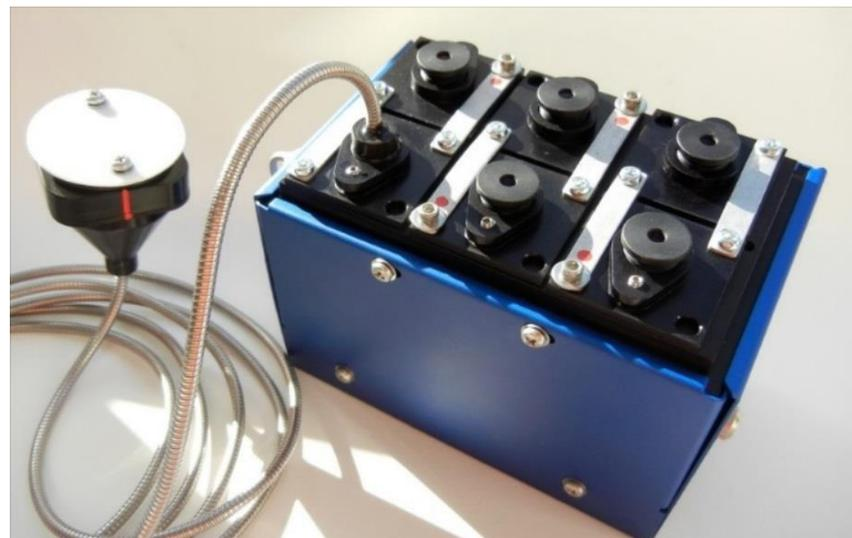
*Tetracam's 6-channel camera with channel 1 attached to a fiber optics.*
