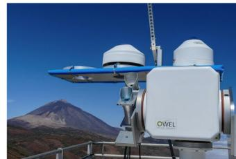
Figure 1.- Pyrgometer Kipp & Zonen CG(R)4 installed on a sun tracker Owel INTRA 3 at Izaña BSRN
