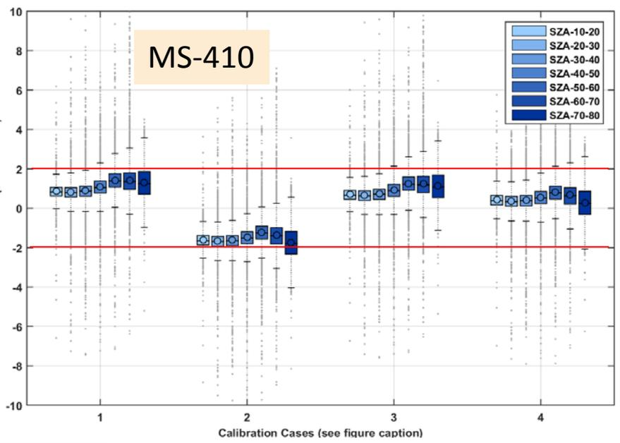
*Indoor and Outdoor calibration comparison between the reference GHI irradiance (using CHP1 for DNI and CM22 for DHI) and CMP22 test radiometer irradiance.*
