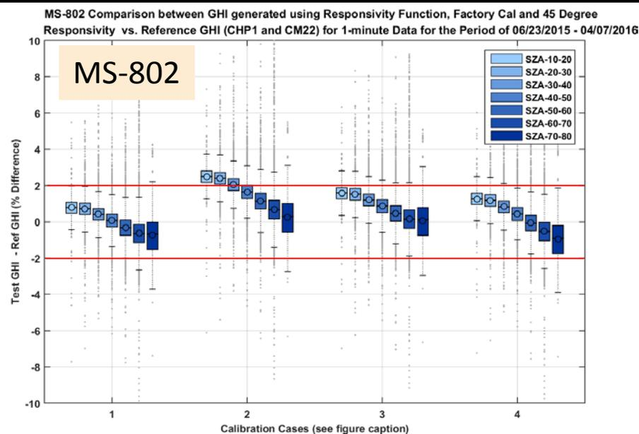
**Indoor and Outdoor calibration comparison between the reference GHI irradiance (using CHP1 for DNI and CM22 for DHI) and CMP22 test radiometer irradiance.**
