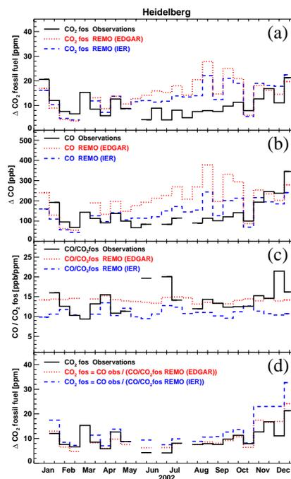
Fig. 2: (a) Fossil fuel  $\text{CO}_2$ , (b) CO, both normalized using  $^{222}\text{Rn}$ , (c)  $\text{CO}/\text{CO}_2\text{fos}$  ratios and (d) fossil fuel  $\text{CO}_2$  recomputed from observed CO and simulated  $\text{CO}/\text{CO}_2\text{fos}$  for two-weekly integrated samples in Heidelberg, comparison of REMO results with observations.
