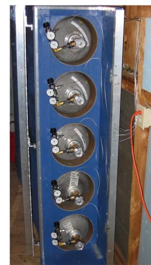
Figure 3: The suite of standard gases installed in the Harvard Forest EMS instrument shack.
