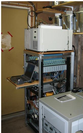
Figure 1: The O<sub>2</sub>/CO<sub>2</sub> analyzer installed in the Harvard Forest EMS instrument shack.
