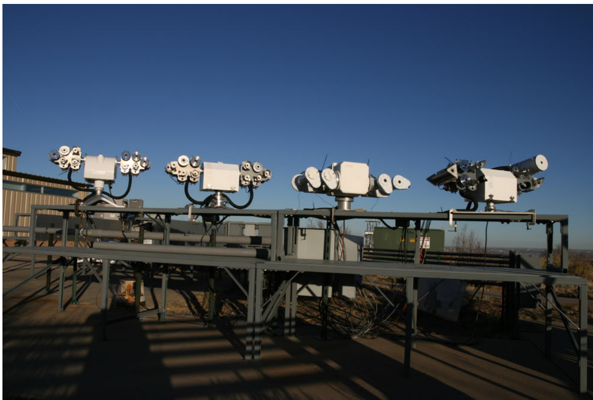
Figure 1. All 33 instruments tracking the sun during the pyrheliometer comparison.
