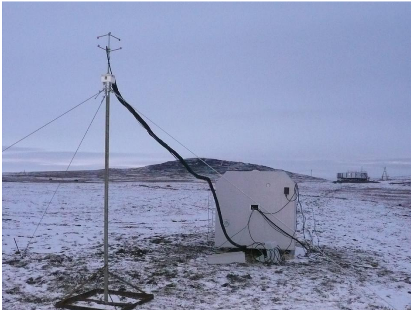
Figure 1. Micrometeorological eddy-covariance fluxes of carbon dioxide and methane are measured on the close-by tundra. Atmospheric concentrations of trace gases and aerosols are measured at the Clean Air Facility on an elevated location behind.
