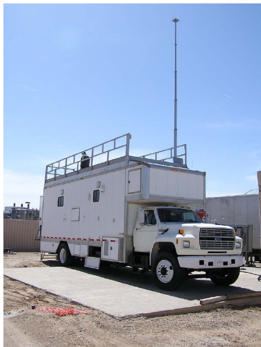
Figure 2. Note the fold-down railings deployed around the top, and the 10 m pneumatic mast.
