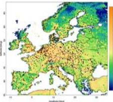
Fig. 1: Locations of 989 feasible towers and masts with a height taller than 100m, using databases from ICOS (existing stations and stations, where location has been decided on), from Wikipedia, and from the European AIS (aeronautical information service) database (EAD). The background map shows CO 2 emissions based on the EDGAR V4.1 inventory at 0.1 deg resolution.
