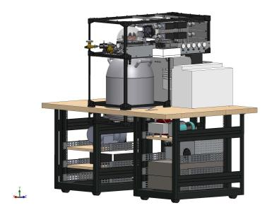
**Figure 1.** GMD's 3-channel GC system under development. Cold-end, vacuum chamber and dewar interfaced to a thermostated chromatographic valve (VICI) enclosure. Transfer lines between the valves and the cryotraps move analytes under helium carrier flow to separation columns in the GC (Agilent 7890) and detectors (MS, FID and ECD).
